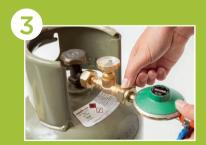
Connect your regulator (not an EFV regulator) to the GasStop and install your hose and device as normal
